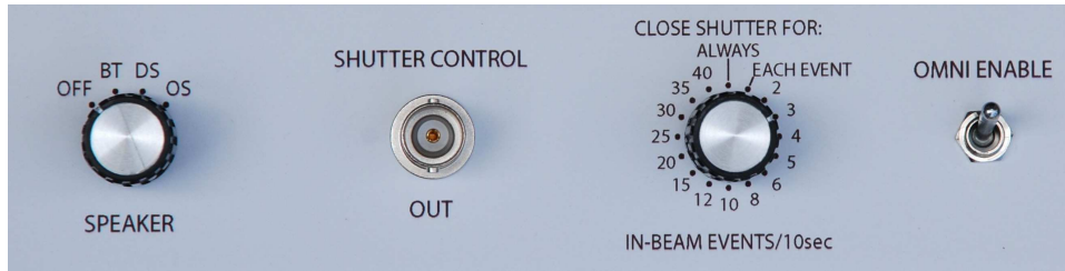
Figure 13: Decoder front panel controls, including the beam sensitivity adjustment and the OMNI enable switch. Here, the system is set for 3 events per 10 s, and the omni logging is enabled. The knob at left controls which signals/conditions the speaker reports.
