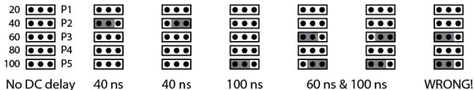
Figure 12: Example lookback jumper configurations for the lookback (DC) delay. If no jumpers are present (or dangling to the side), then this action is effectively disabled. A single jumper can occupy any delay from 20–100 ns in either the left or right columns. Up to two jumpers can be used for a combined effect, but only if their columns differ. The last example to the right is invalid.
