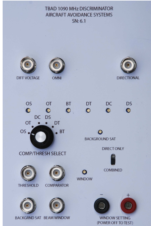
Figure 5: Discriminator box front, where threshold adjustments are made. The knob selects which threshold is made available to the THRESHOLD BNC, with trimpots labeled accordingly. Signals from the two RF power detectors are available, as is the differential amplifier (gain = 4) output. The various comparators associated with the six thresholds may also be monitored at the COMPARATOR connector, likewise knob-selectable. One may also adjust and monitor window width and background saturation duty cycle from the front panel. Finally, one may select whether transmitted DATA is based on directional signal (DT) alone, or combines omni (OT) as well.
