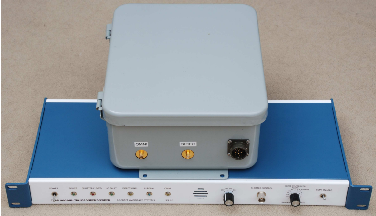
Figure 2: Discriminator box (top) and decoder box (bottom). The discriminator box is contained within a weatherproof shell, and has connectors for the two antenna signals and for the umbilical to the decoder box (carries power and communications).
